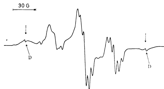
Fig. 6. ESR spectrum of \text{CH}_2\text{DND} radical on PVG. Arrows: \longleftrightarrow D, D atom; \longleftrightarrow , hump
