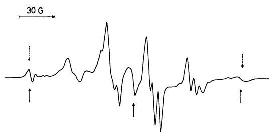
Fig. 2. ESR spectrum of \text{CH}_3\text{ND} radical on PVG. Arrows: \longleftrightarrow , \text{CH}_2=\text{N} radical; \longleftrightarrow , hump
